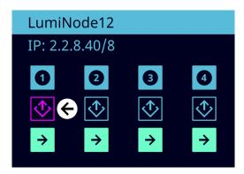
If the port is in DMX redundant mode and active the output icon is solid magenta: 🌣
