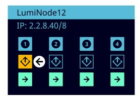
To clear to warnings, scroll to the following display and press the jog wheel. This screen can be found when scrolling left once when ports 1-4 are shown or to scroll all the way to past the last detailed port info.
