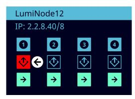
If the lost stream is recovered the LCD display will show this by changing the Output orange.
