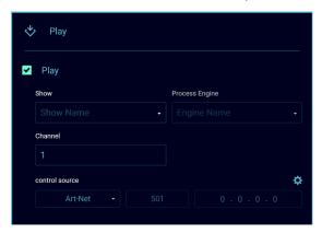
Select the control channel you want to use to control the cue list. Use the cog wheel to set the source protocol and universe and if required a specific controller IP.
